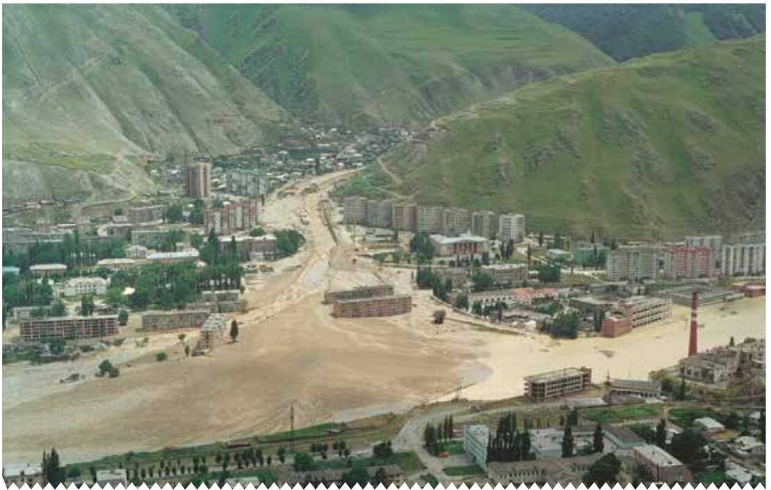
Figure 6: Debris flow originating from glacial moraines/till above the town of Tyrnauz, Russia, July 2000. The most probable trigger of the debris flow was considered to be an outburst from an englacial cavity (Photo: A. Aleinikov).
