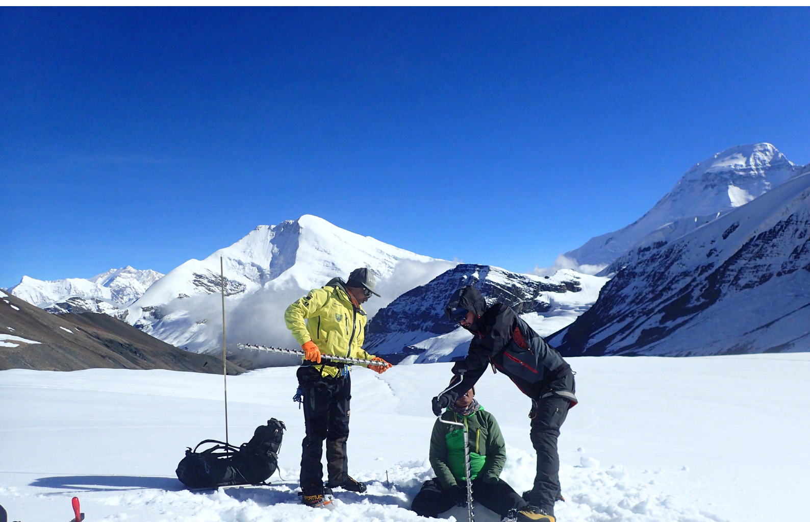
Installation of mass balance stakes on Rikha Samba Glacier, Nepal (Photo: Jakob Steiner)
